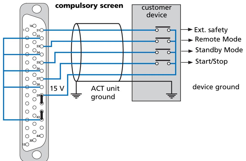
The voltage used to power the contacts is supplied by the ACT 600 TH (terminals 39-40). The disadvantage of this method is the risk of exposing this voltage to external interference (see also diagrams on page 1/5).
