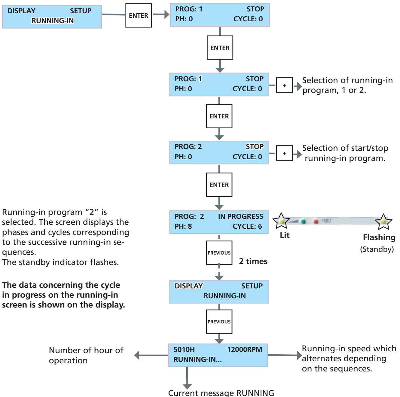
Running-in program "2" is selected. The screen displays the phases and cycles corresponding to the successive running-in sequences. The standby indicator flashes.
